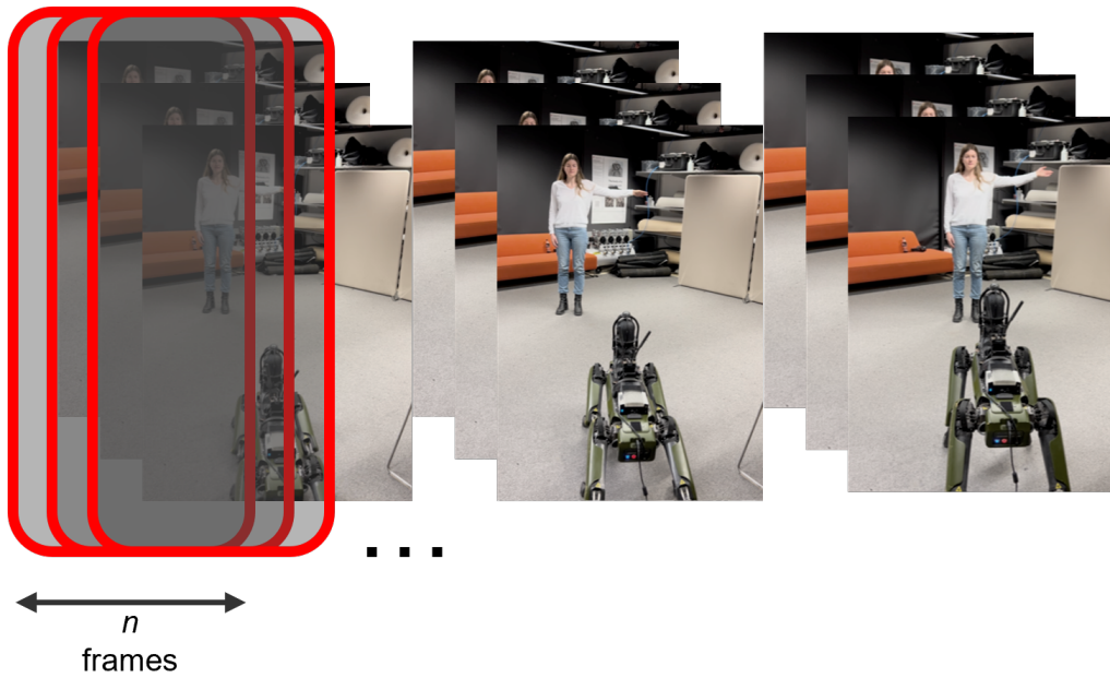
Figure 4.10: Sliding window protocol. The full input frame sequence is split into shorter sequences.
