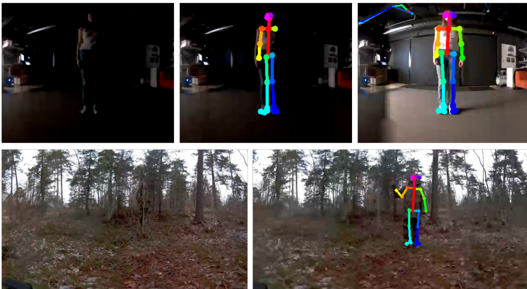
Figure 4.4: The top row shows how OpenPose performance improves with better illumination. Bottom left, the person wears camouflage clothing and is partly obscured by a small tree.
