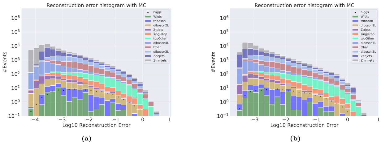
Figure 4.1: Reconstruction error on validation SM MC from the small (a) and large (b) autoencoders. The Higgs channel has been removed from training and is used as signal. No significant difference in distributions is found.
