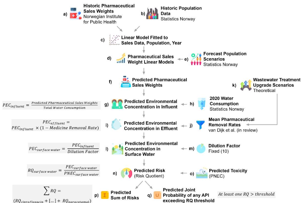
Figure 12: Diagram of data sources, workflow, equations, and output of Paper III. Historic pharmaceuticals sales (a) for 6 Active Pharmaceutical Ingredients (APIs) and population (b) are fitted to a linear model (c), which is then used (d) with a range of population forecast scenarios (e) to predict sales weights (f). These sales weights are subsequently used to calculate Predicted Environmental Concentrations (PECs) in influent (g), based on 2020 water consumption figures (h). PECs in effluent (i) are calculated across various wastewater treatment upgrade scenarios (k) using abstracted removal rates (j), and a PEC in surface water is calculated (l) using a fixed dilution rate of 10 (m). Risk Quotients (RQs) are then predicted, per API and scenario (n), using externally sourced toxicity data (o). Finally, a predicted sum of RQs (p), and the joint probability of RQs exceeding various thresholds (q) were calculated across the APIs for each scenario. Reproduced from Welch et al. (preprint, 2023)
