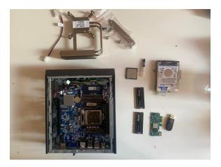
Figure B.3: Shuttle XH110G Components
