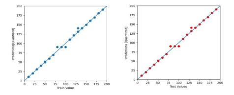
Figure 5.12: Quantized CNN's training and testing prediction compared to the true values.
