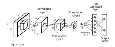
Figure 2.8: Convolutional Neural Network with Fully connected Layer
