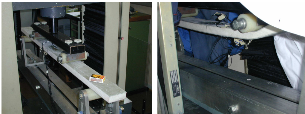
(a) The sandwich beam and bearings before the load is applied. (b) The indentation of the core under the load-bearing.
