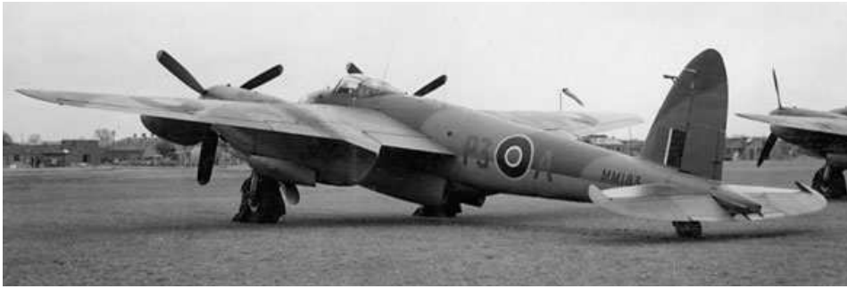
Figure 1.1: A Mosquito Bomber from World War Two. Known as the first mass produced airplane using sandwich panels.
