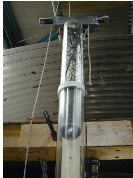
(b) Projectile and wire ready for the next impact test
