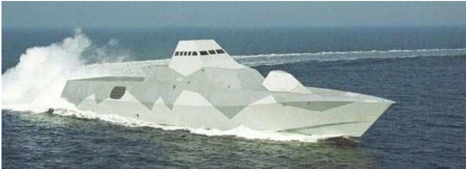
Figure 1.3: A Visby stealth corvette. The hull material is a sandwich construction comprising a PVC core with a carbon fibre and vinyl laminate.
