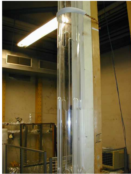
(a) Air holes in the tube, allowing the air to flow out of the tube during impact.
