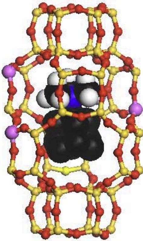
**Figure 4:** CHA cage with template
