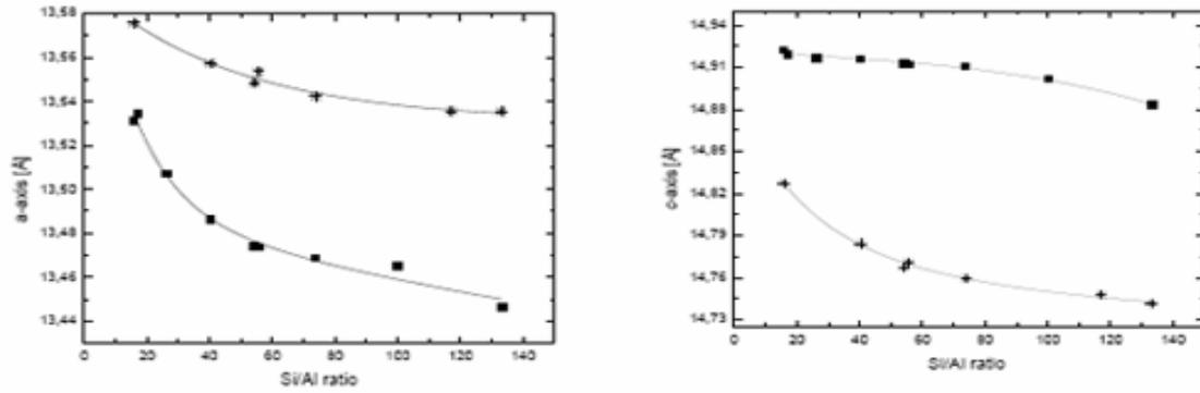
**Figure 3:** Unit cell parameters for as-synthesized samples (square) and for calcined samples (star) as a function of the Si/Al ratio
