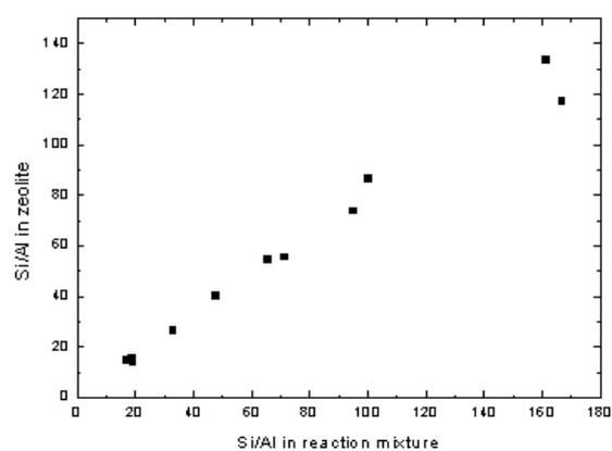
**Figure 2:** Si/Al ratio in the materials determined by ICP-AES as function of the Si/Al ratio in the reaction mixture
