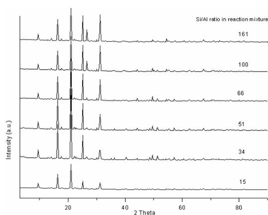
**Figure 1:** Diffractograms of samples with different Si/Al ratio
