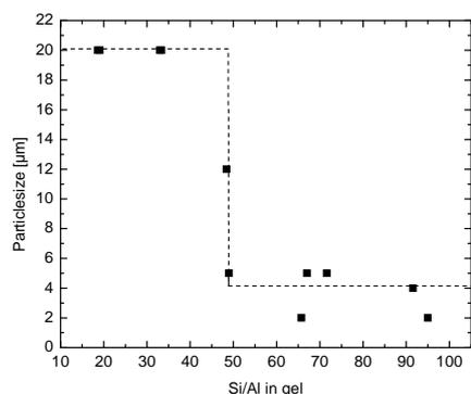
**Figure 5:** Particle size as function of the Si/Al ratio in the reaction mixture
