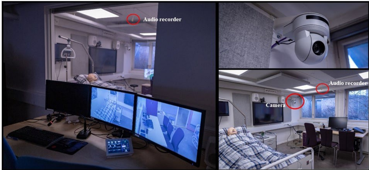
Figure 4: The control room and camera and audio placement
