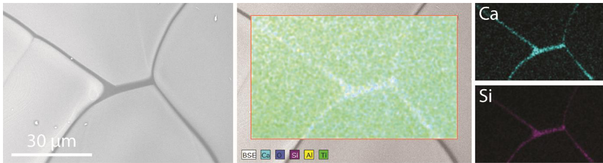
Figure 3-9: EDX mapping is used to investigate elements present within the sample. While Ti is highly concentrated within the grains, Ca and Si are highly concentrated in the grain boundaries.
