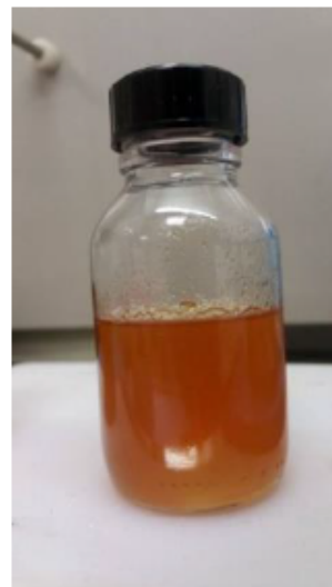
Figure 1: A BG-PCL hybrid solution. Its translucency indicates that the organic and inorganic phases are homogeneously mixed.
