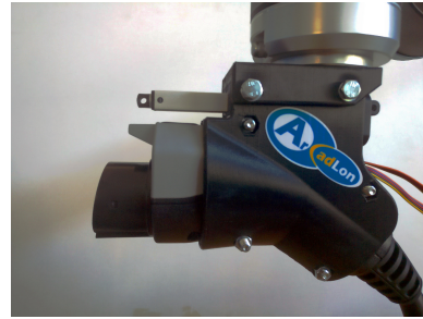
Fig. 5. Custom 3D printed connector plug holder attached to the end-effector of the UR10 robot.
