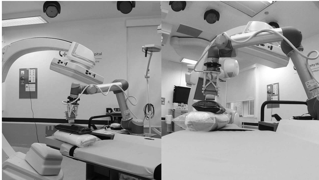
Figure 1.1. UR5 robot holding an ultrasound probe over a dummy patient next to a C-arm mounted fluoroscopy scanner. Photo taken in Oslo University Hospital.
