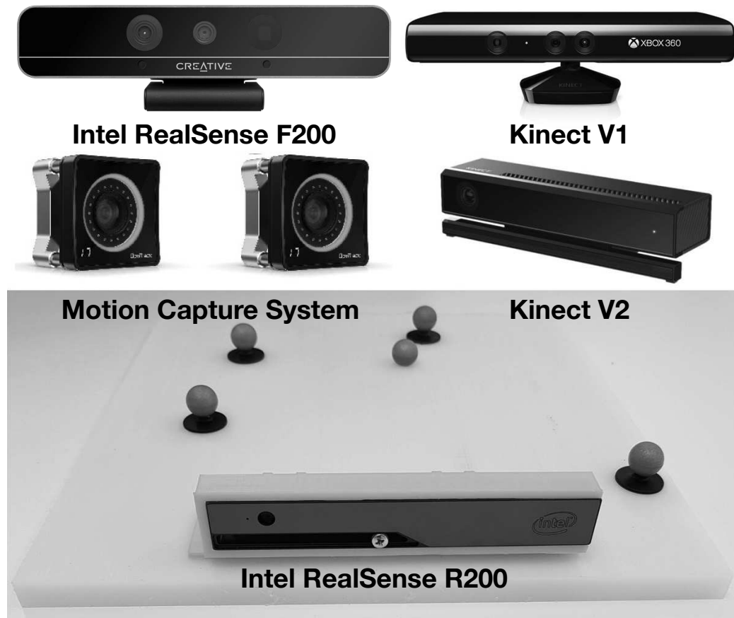
Figure 2.2. Vision sensors used in the projects: 3D cameras and Optitrack motion capture system.
