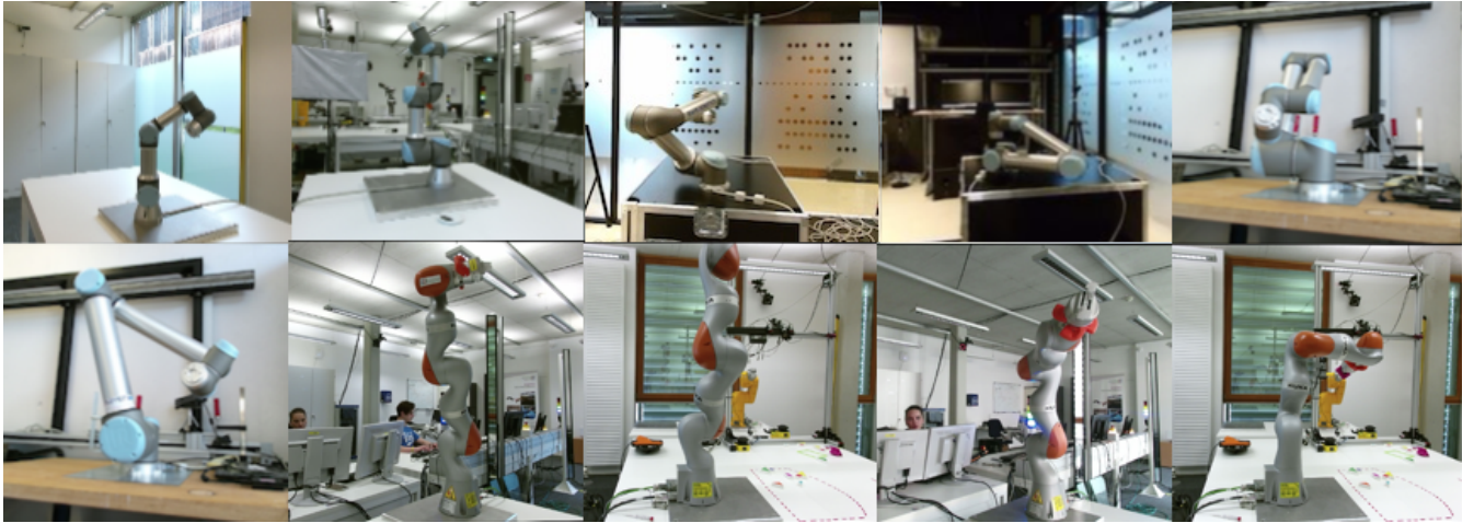
Fig. 1. Samples from the collected robot datasets. It consists of a line of Universal Robots (silver-blue) as well as Kuka LBR iiwa (silver-orange). The data was collected with a variety of backgrounds and light conditions to provide more robustness.
