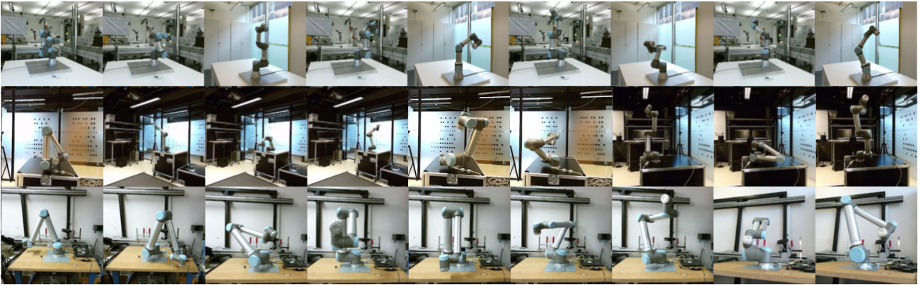
Fig. 1. Samples from a collected robot dataset. Each row of images represents different robot type in the following order: UR3, UR5 and UR10. The dataset was created using a varying background to provide more robustness.
