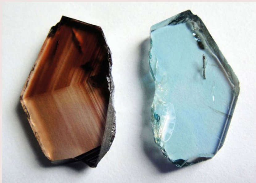
Figure 6: These two slices were cut from a gem-quality zircon crystal from Phnum Trom (largest dimension 17 mm). The samples were prepared as doubly polished plates (2.7 mm thick), and the half on the right was subjected to heat treatment whereas the one on the left remained in its initial state. The untreated specimen shows strong zoning, which disappeared after heat treatment. Photo by Astrid Wittwer.
