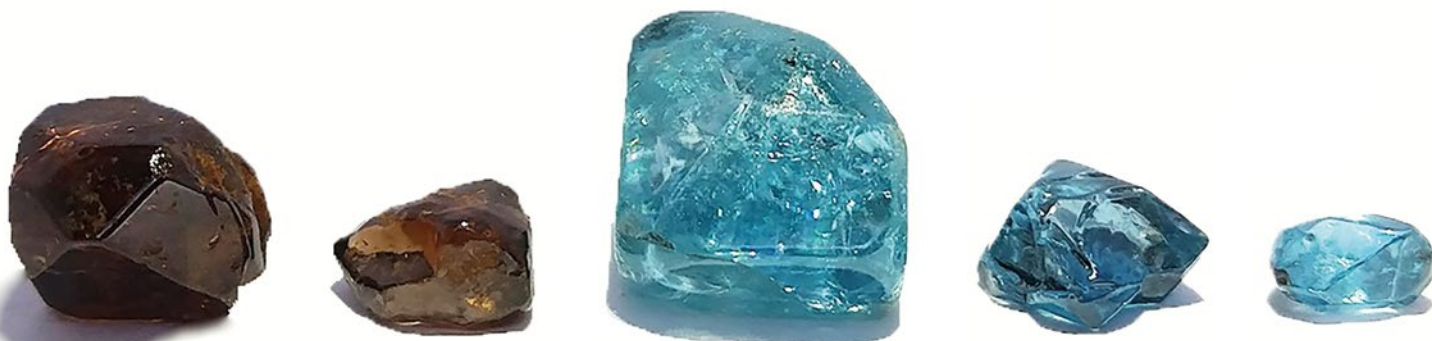
Figure 4: These zircon samples from Ratanakiri (0.3–5.1 g) include two untreated brown crystals and three blue specimens that were heat treated at ~1,000°C under reducing conditions for a few hours. Photo by M. Zeug.
