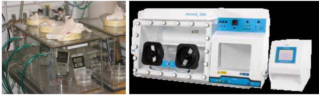
Figure 5. Custom made hypoxia chamber (left) and hypoxia chamber Invivo 500 from Thermo Scientific (right)
