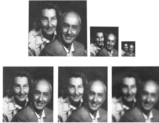
Fig. 2.13 Adelson's pyramid structure, known also as Gaussian pyramid. On the top, the original image and the sequence of two subsampled images. On the bottom, the levels are expanded to the size of the original image and the effects of the filtering are clearly apparent. Figure extracted and reproduced from the original paper by Adelson et al. [2].
