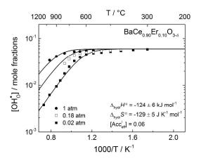
Figure 3: Equilibrium proton concentrations measured by TG of all compositions investigated given in the following order; BCSc10, BCY10, BCIn10, BCGd10 and BCEr10. The solid lines are the curve-fitted proton concentrations.
