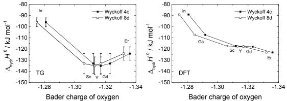
Figure 7: Hydration enthalpies evaluated by curve-fitting TG curves (left) and by DFT calculations (right) plotted as a function of the oxygen Bader charge closest to the dopant. Bader charges have been determined by DFT calculations.
