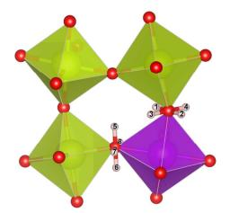
Figure 1: Schematic of eight of the proton positions around the dopant investigated for all acceptor doped  $BaCeO_3$  supercells. The yellow octahedra are  $CeO_6$  while the purple octahedron is  $GdO_6$ . 1-4 depict positions around the O4cx while 5-8 depict positions around O8dx.
