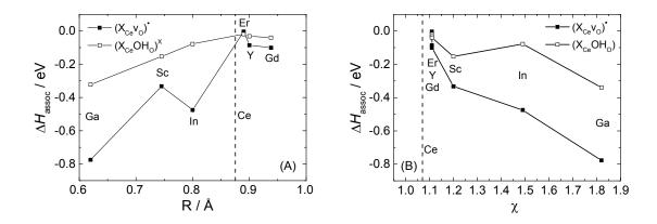
Figure 5: Association enthalpies between the acceptor and oxygen vacancies or protons calculated by DFT as a function of ionic radius (A) and electronegativity (B) for the acceptor.
