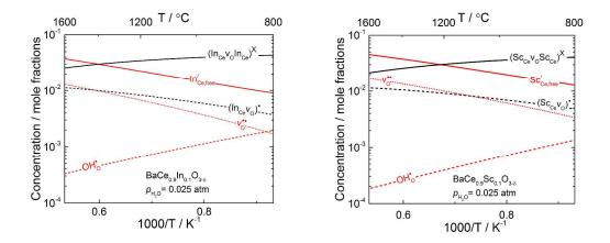
Figure 8: Equilibrium defect concentrations for all defects considered in this work for BCIn10 and BCSc10 using thermodynamics determined by DFT calculations as a function of temperature under wet conditions ( $p_{\rm H_2O} = 0.025$  atm).
