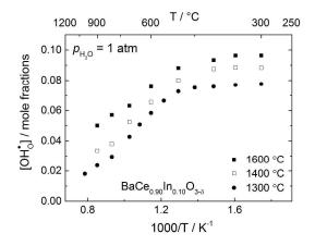
Figure 9: Equilibrium proton concentrations determined by TG for three different samples of BCIn10 calcined at 1300, 1400 and 1600 °C for 12 hours.
