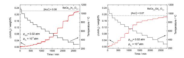
Figure 2: Thermogravimetric (TG) measurements of the water uptake for BaCe<sub>0.9</sub>In<sub>0.1</sub>O<sub>3- $\delta$ </sub> (BCIn10) (left) and BaCe<sub>0.9</sub>Gd<sub>0.1</sub>O<sub>3- $\delta$ </sub> (BCGd10) (right). Both measurements have been conducted in wet Ar ( $p_{O_2} = 10^{-5}$  and  $p_{H_2O} = 0.02$  atm) and have been corrected with a blank run where the alumina crucible was empty.
