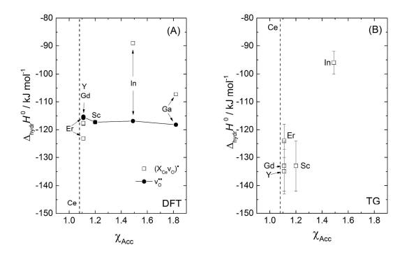
Figure 6A: Hydration enthalpies of unassociated and associated oxygen vacancies, closed and open symbols, respectively, as calculated by DFT as a function of the electronegativity of the acceptor. B displays the hydration enthalpies determined experimentally from TG measurements for comparison. The dashed line indicates the electronegativity for Ce for reference.
