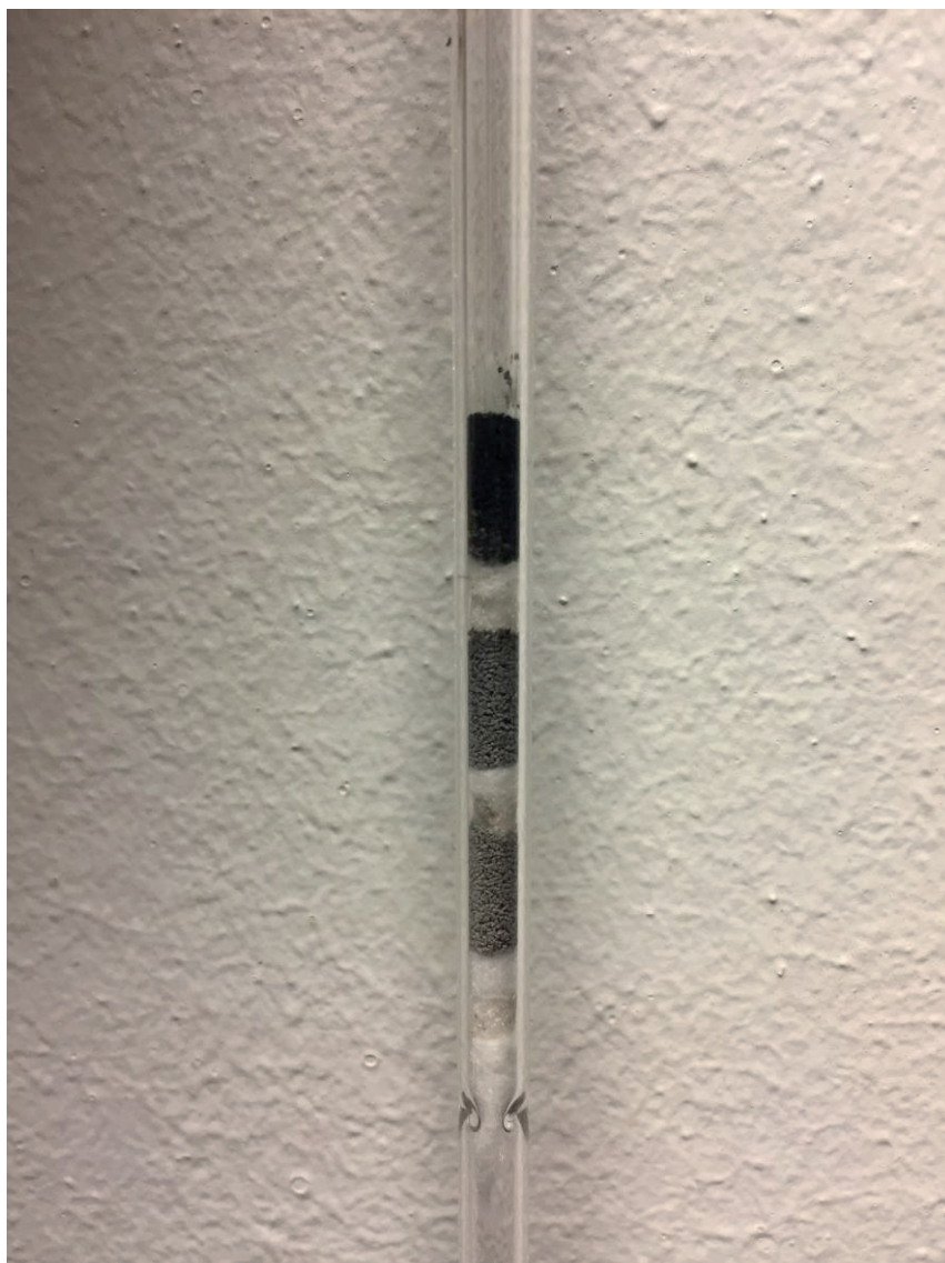
Figure A-1. Photograph of the ZSM-5-MFI-27 bed after running the MTH reaction at 400 °C, WHSV = 2 \text{ g}_{\text{MeOH}} \text{ g}_{\text{cat}}^{-1} \text{ h}^{-1} and P_{\text{atm}} for 7 hours. The black area corresponds to the top layer, the dark grey zone is the middle layer, and the light grey area corresponds to the bottom layer.
