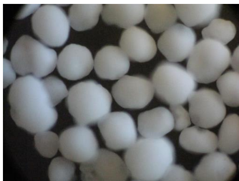
Picture 1. Spray granulated 30:70 (w:w) triglyceride: \beta -CD powder. The oil contained 60% (w/w) triglycerides. (10x magnification)
