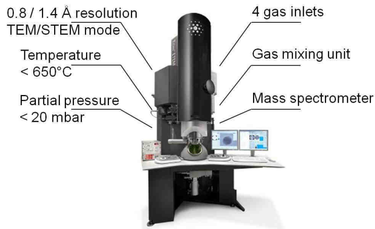
Figure 4.5 Illustration of the Titan 80–300 ETEM microscope and its in situ units (adapted from [81]).
