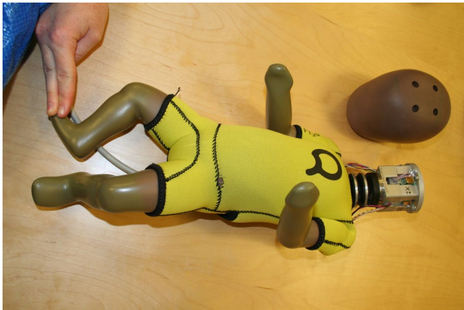
Figure 2.7.3: The crash test dummy with the accelerometer bracket.
