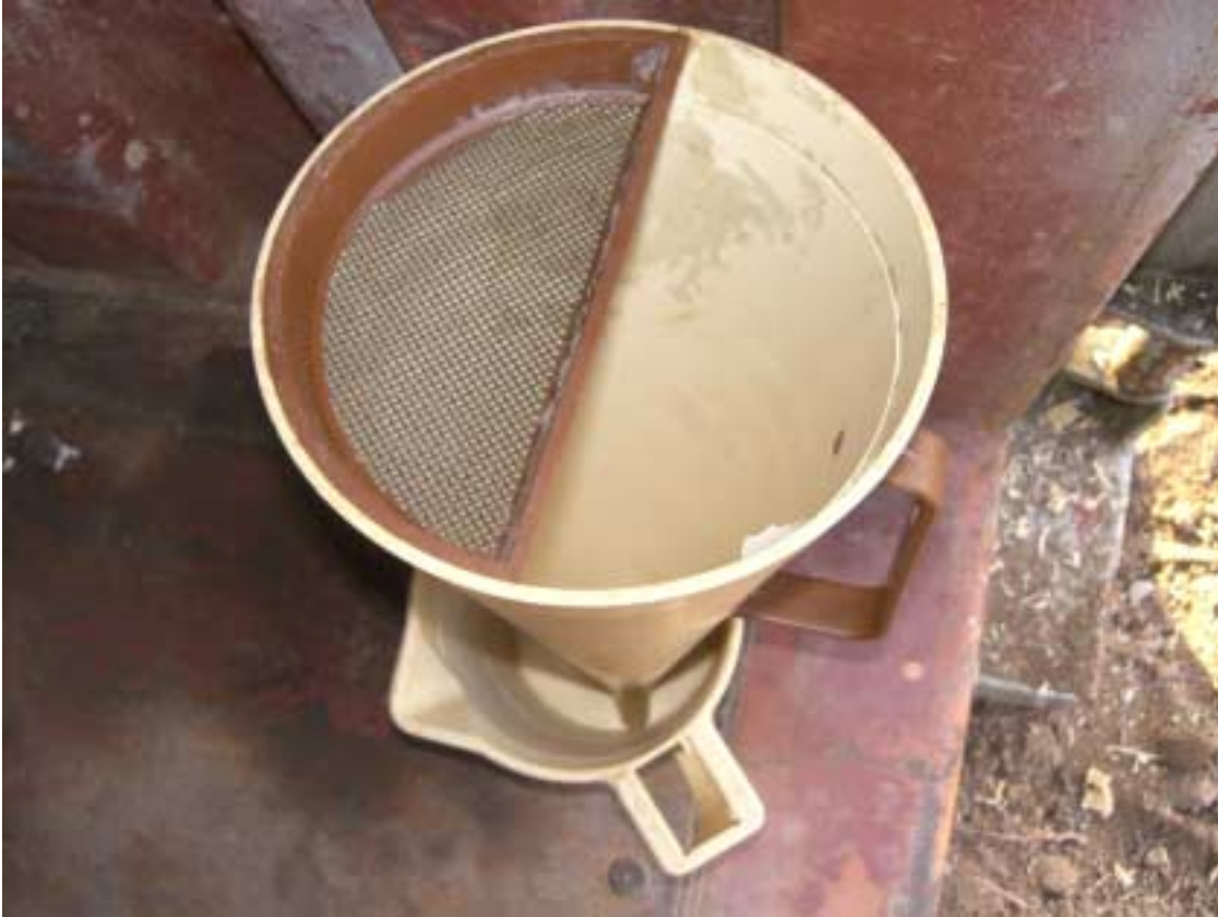
Figure 3.8: Marsh funnel showing the pouring mesh side. The mesh side used to filter the mud so that the outlet can not be blocked.
