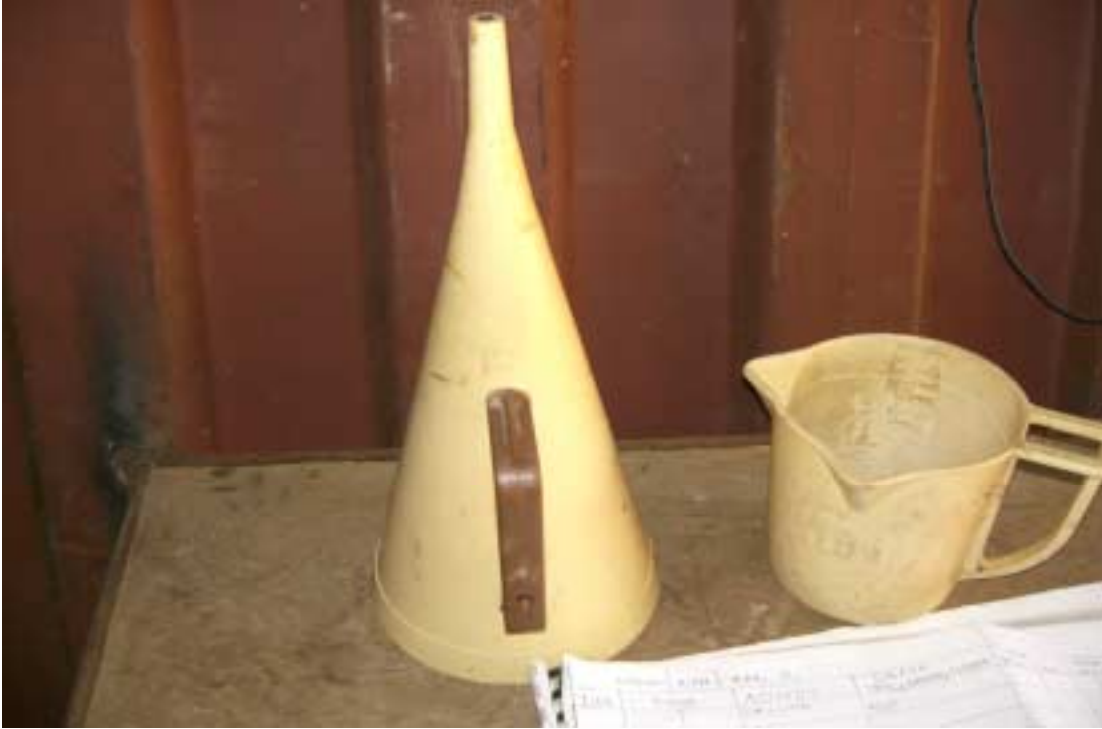
Figure 3.7: Marsh funnel used at the site to determine the mud viscosity
