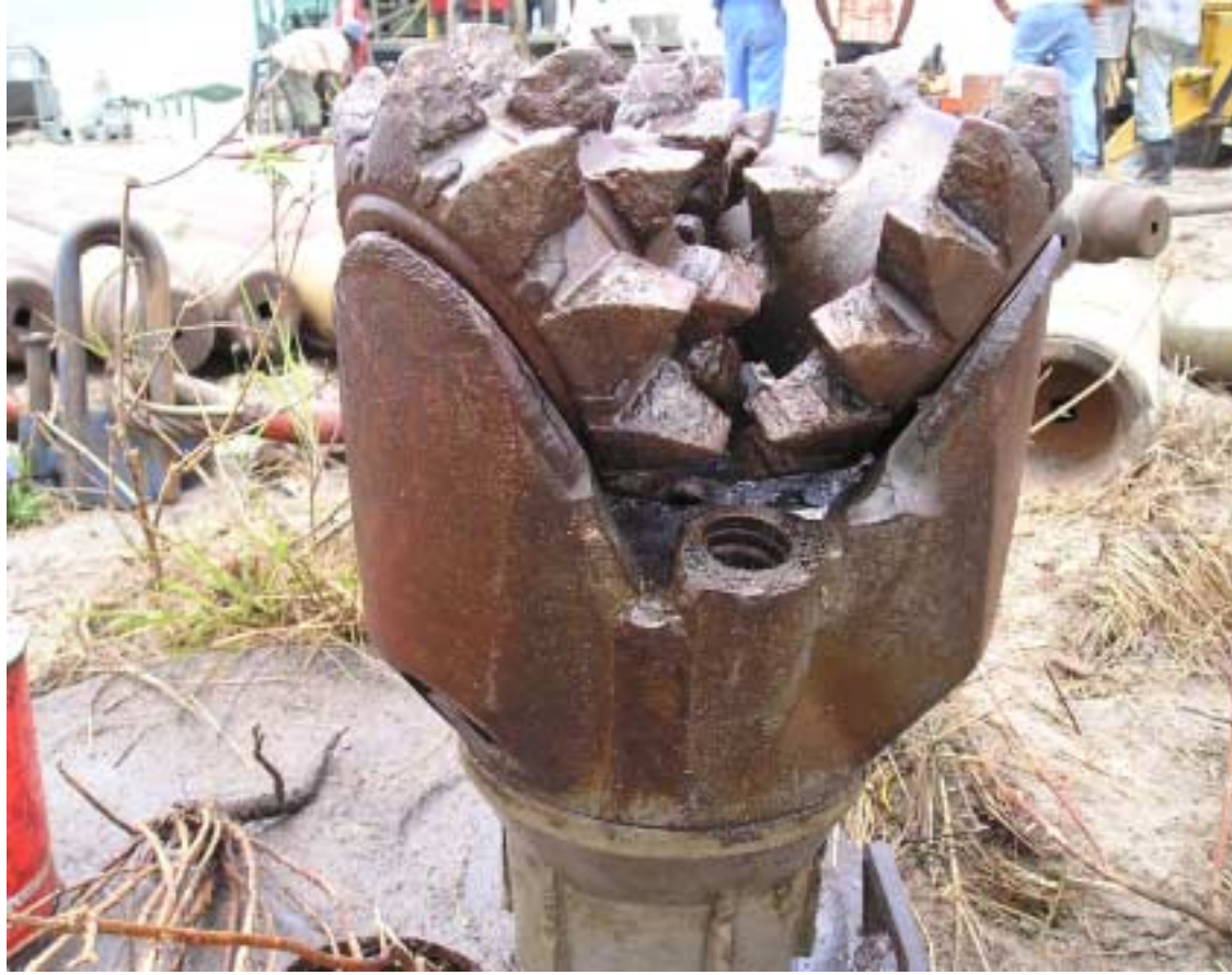
Figure 3.2: Roller bit applied at Kimbiji site. The diameter of the bit is 311 mm.
